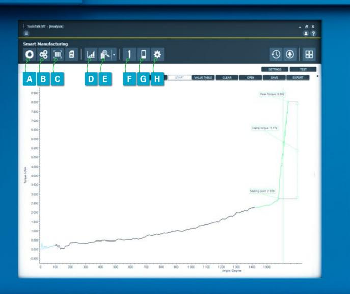
**F TOOL SETTINGS**: Keep track of the quality of your tools, by analyzing the tool lifetime performance and setting calibration intervals.
